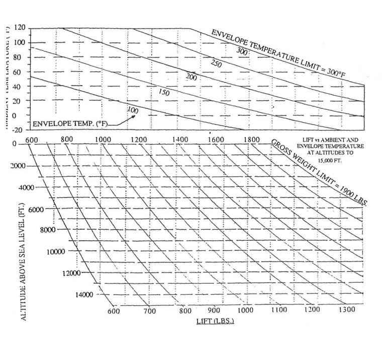
Figure 1 shows the effect of varying conditions on the lifting capability of a fully inflated Firefly 8B-15 envelope.
